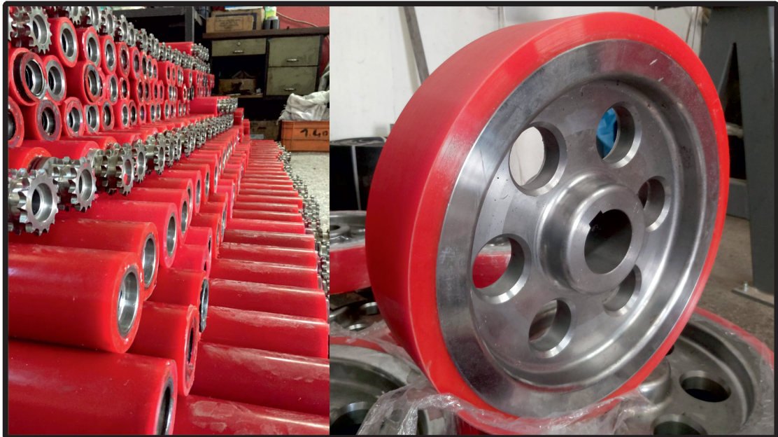
Poliüretan Kaplama | Polyurethane Coating
